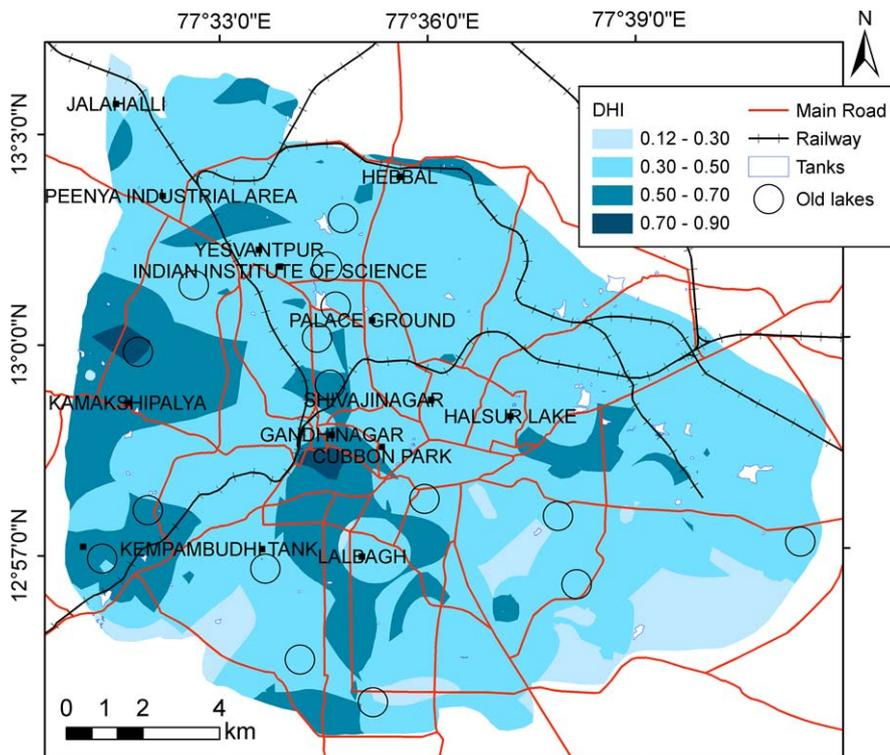
**Fig. 9.** The deterministic seismic hazard microzonation map of Bangalore city; the listing of old lakes (reclaimed lands) have been given in caption of Fig. 8.
