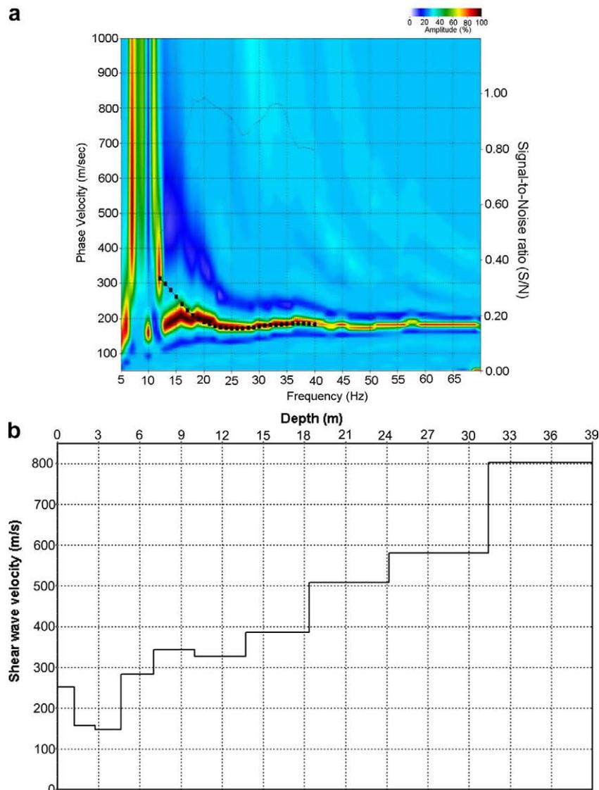
Fig. 5. Typical results from multi-channel analysis of surface wave (MASW) survey for the study area: (a) dispersion curve and (b) shear-wave velocity profile.
