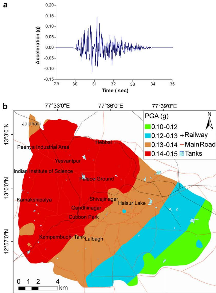
**Fig. 2.** (a) A representative accelerogram generated through stochastic modeling at bedrock level, and (b) the deterministic spatial distribution of peak ground acceleration at bedrock level depicting a variation from 0.10 to 0.15 g in the Bangalore city.
